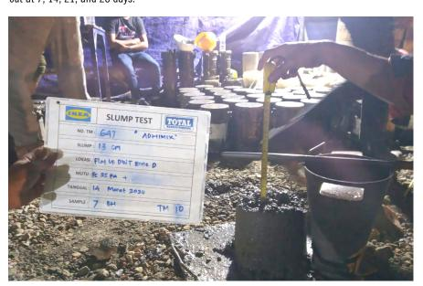
Slump test after addition of Xypex Admix
