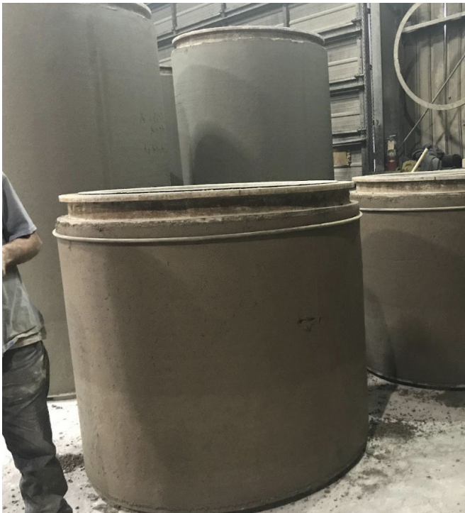
The new precast concrete pipes containing Xypex for the upgraded East Lansing sewer system.
