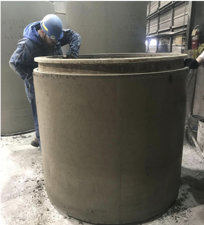
Xypex Bio-San used in precast concrete of sewer systems for permanent waterproofing and corrosion protection.
