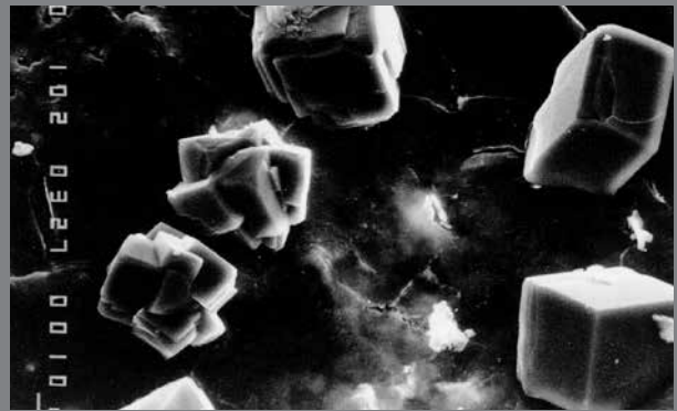
UNTREATED CONCRETE AT 50 MM
