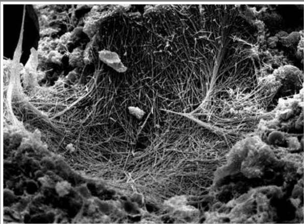
XYPEX TREATED CONCRETE
